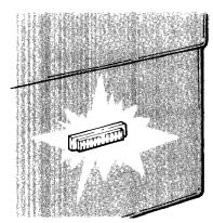
Exterior signal light — located on the right front of the freezer at the bottom, the signal light automatically warns of any unexpected power failure. When power is being supplied the light will glow. If light does not glow, check immediately. The electric current may be off; the freezer may be disconnected from the outlet; or the warning light may be burned out.
